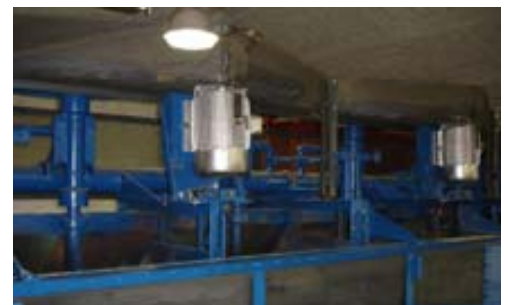
Primary Floatation Cells in Main Mill Building as Shown in a February Photo Gallery Update
