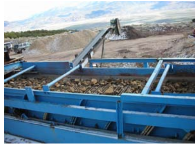
Material moving through the screening plant
